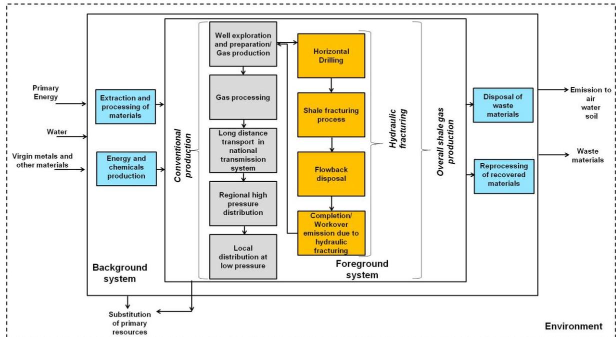
Figure 1. System boundary for shale gas. Yellow boxes represent the hydraulic fracturing process, grey boxes identify the conventional processes and the blue boxes refer to the activities of the background system.
